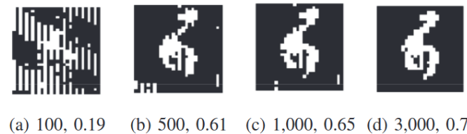
Fig. 10: Recovered images for the ZCU104 board for (number of runs, normalized cross-correlation with the original image).
